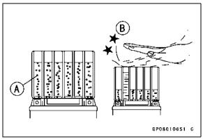
Keep the container in place for 20 minutes or more. Don't remove the container from the battery until it's empty, the battery requires all the electrolyte from the container for proper operation.
